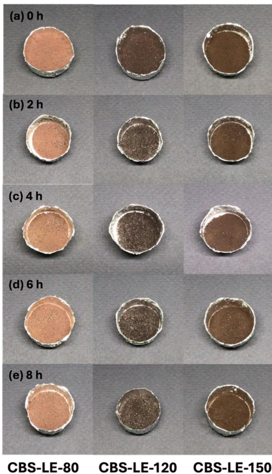
Figure 5 The color of lignin extracts prepared from cocoa bean shells (CBS) at temperatures of 80 °C (CBS-LE-80), 120 °C (CBS-LE-120), and 150 °C (CBS-LE-150)
