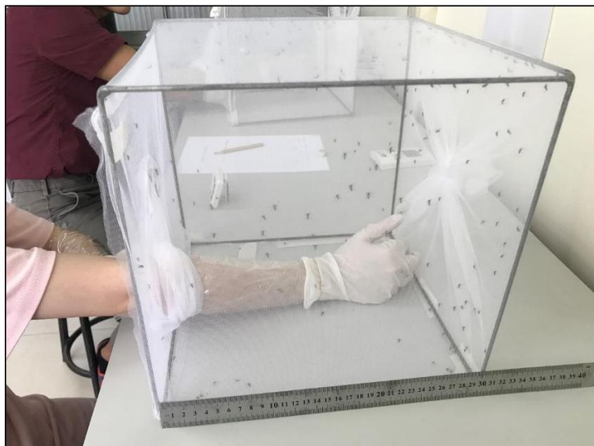
**Figure 3.** Mosquito repellency testing with *Ae. aegypti* by “arm in cage” test according to the WHO standard method.
