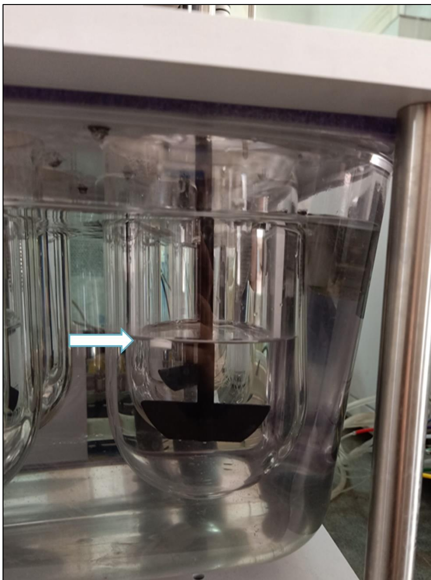
Figure 5. A photograph taken during in vitro drug release studies of F1 in 0.1 N HCl.
