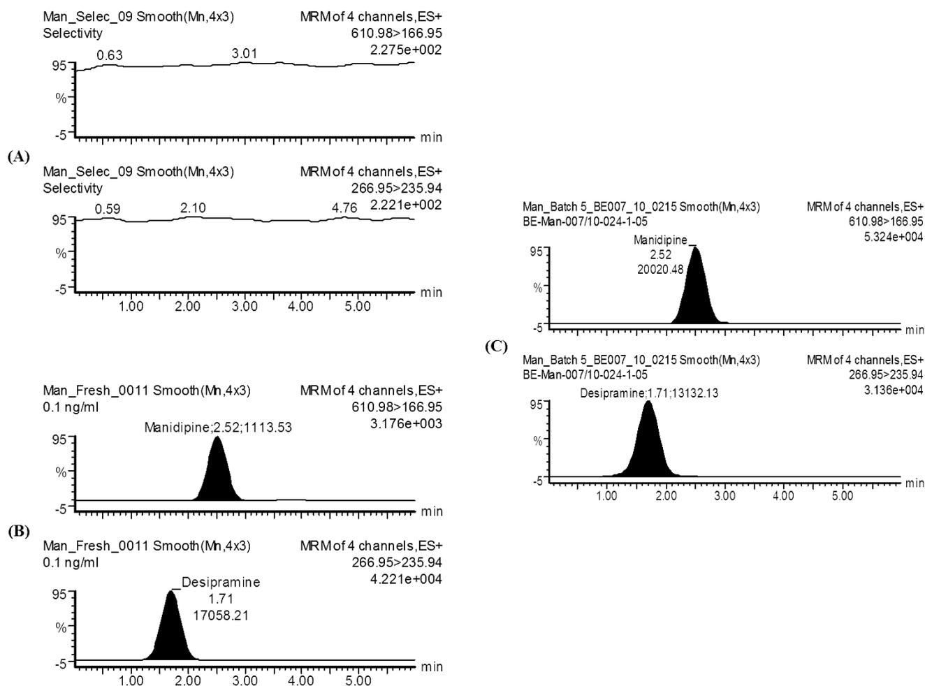
**Figure 3.** The chromatogram of extracted drug free human plasma (A), LLOQ sample at 0.1 ng/mL (B) and clinical plasma sample at 1.5 h after an oral administration of 20 mg manidipine hydrochloride tablets (C)
