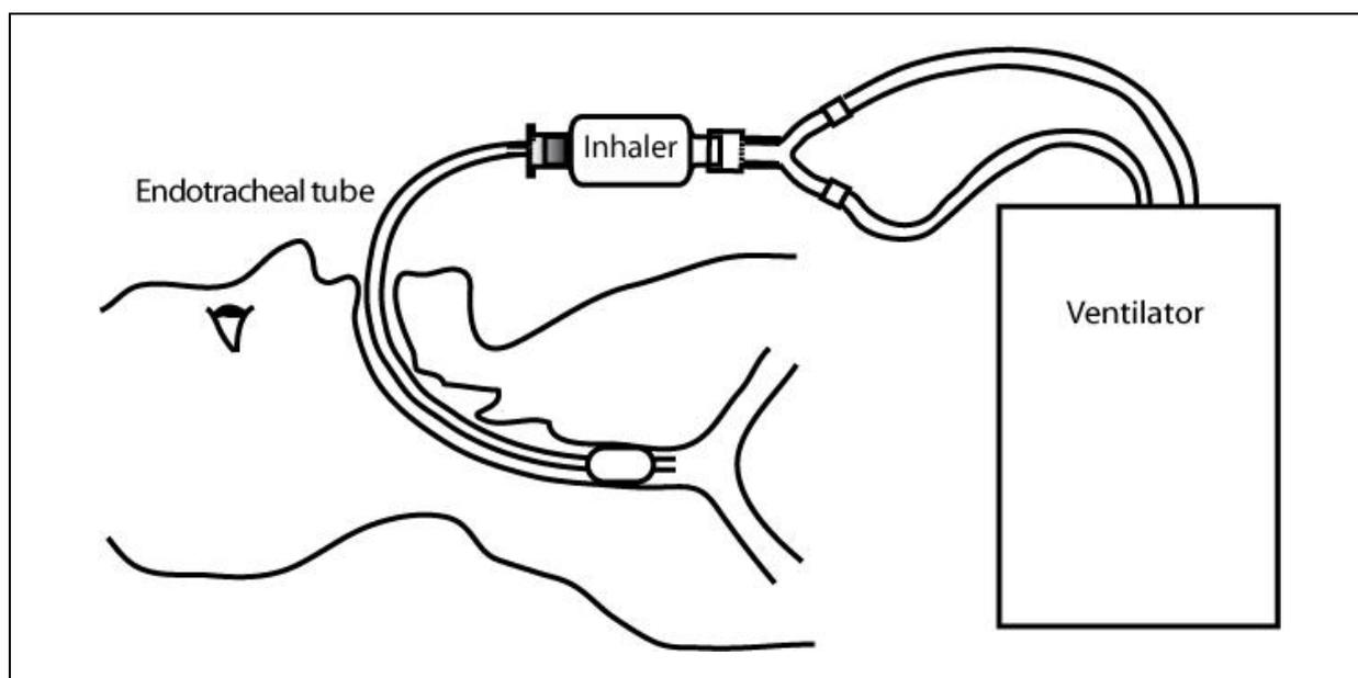
**Figure 2.** Direct connection of an inhaler device within the ventilator circuit. Here, the inhaler is placed between the ventilator tubing and the endotracheal tube. Aerosols may be generated using an external energy source (e.g. ultrasound) or by utilizing the energy supplied by the ventilator.
