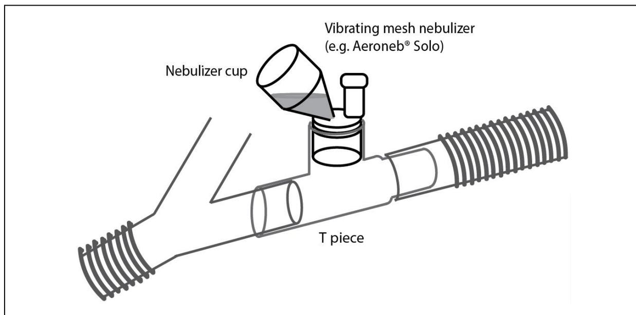
**Figure 1.** Aeroneb<sup>®</sup> Solo, a vibrating mesh nebulizer, in ventilator circuit.
