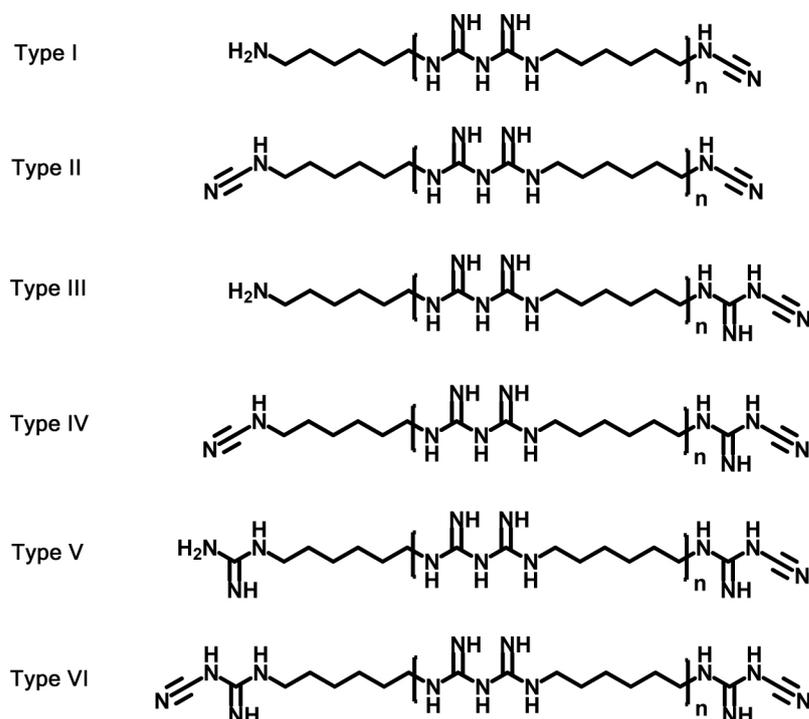
**Figure 2.** Typical structures reported in the literature [10] for polyhexamethylene biguanide.
