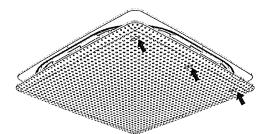
Push the middle grille fixture to unlock the suction grille first and followed by the side fixtures.
