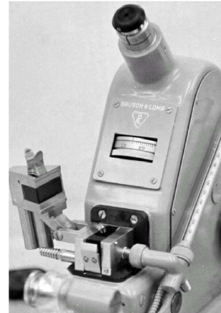
Fig. 2-6. Typical classical Abbe refractometer opened to show prism system.
